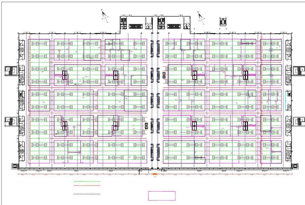
Fig. 4 – Figure showing the lines of purlins in pavilions 16 and 20. The points marked in green are the positions that can be used to support the vertical structures of a raised platform, while the points marked in red are the positions which cannot be used. The blue marks show the lines of trusses supporting the purlins, while the perimeters of the stands are marked in maroon.
