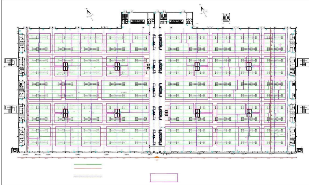
Fig. 3 – Figure showing the location of the lines of purlins in pavilions 8 and 12. The points marked in green are the positions that can be used to support the vertical structures of a raised platform, while the points marked in red are the positions which cannot be used. The blue marks show the lines of trusses supporting the purlins, while the perimeters of the stands are marked in maroon.
